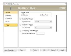
Point Mode). The device can take as many as 380,928 readings with both channels enabled and 419,020 pressure only readings. The data logger will record up to 50 samples of "pre-trigger" data.
